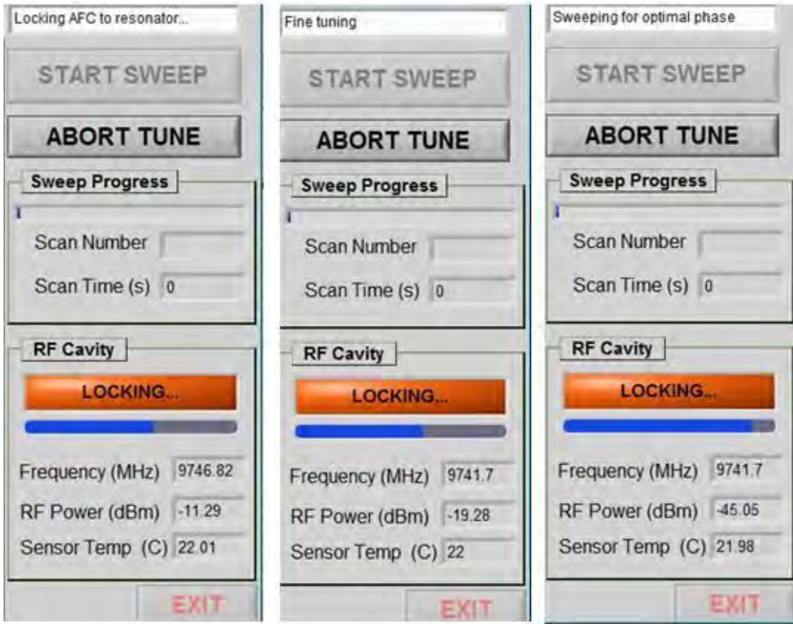
Figure 6.7: Locking the AFC to the Resonator, Fine Tuning, and Sweeping for Optimal Phase.
