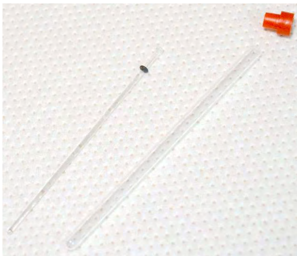
Figure 7.4: O-Ring Used to Keep the Smaller Tube Aligned Inside the 5 mm Tube
