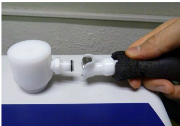
Figure 10.7: Attaching the Air Hose from the ThermoCube via CPC Adapter to the Air Flow Adapter (shown with cover)
