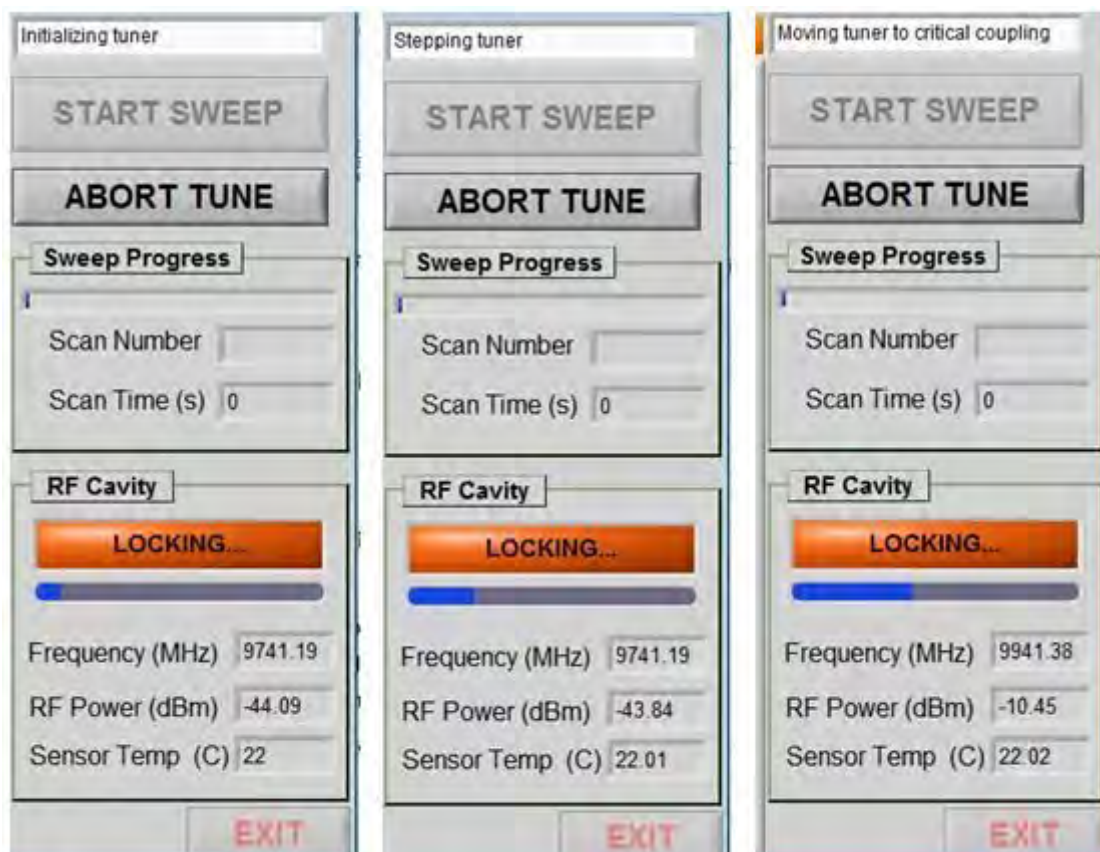
Figure 6.6: Initializing the Tuner, Stepping the Tuner, and Moving Tuner to Critical Coupling.
