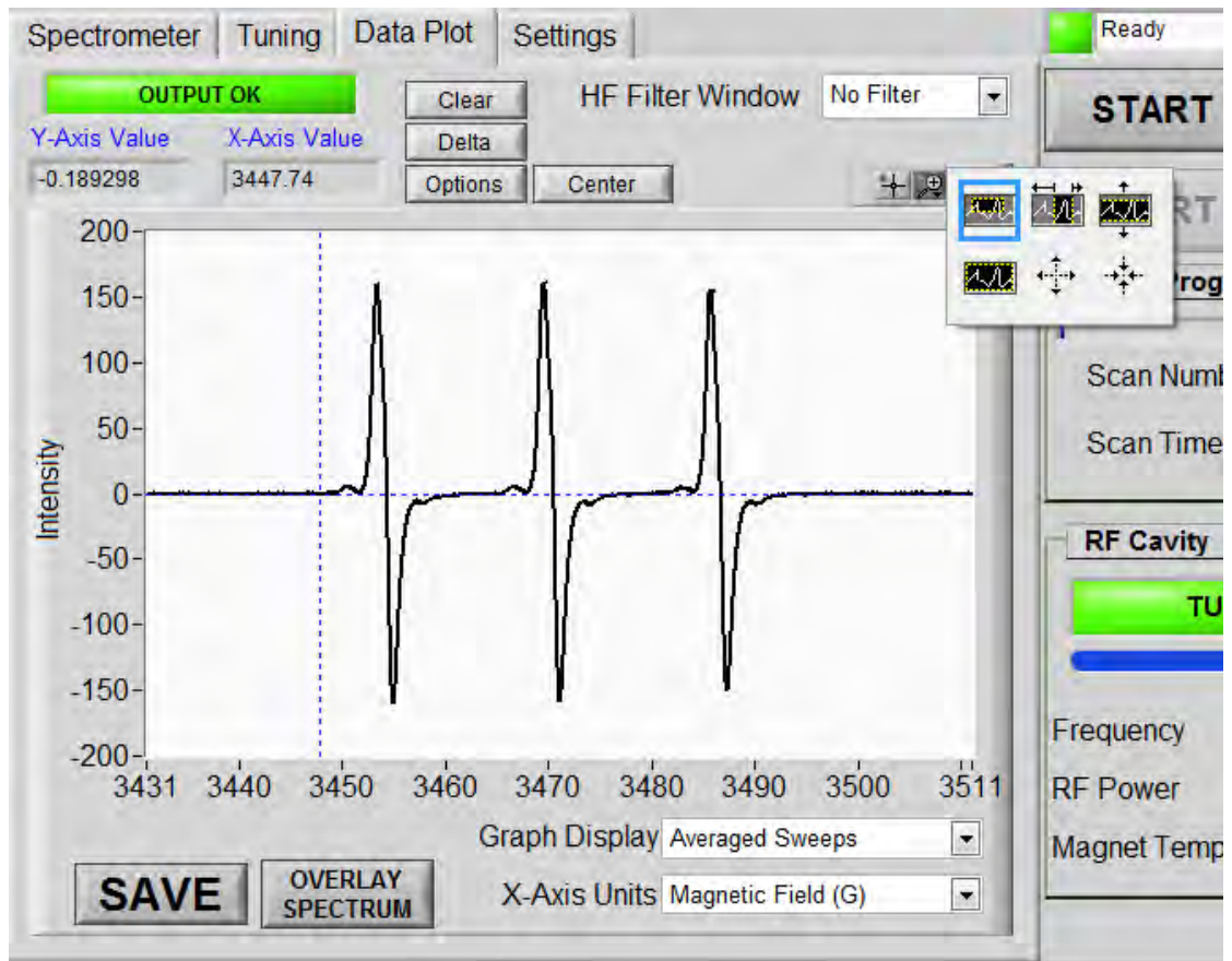
Figure 8.44: Pop-up displayed when the center icon is selected. Select upper left icon to expand spectrum.
