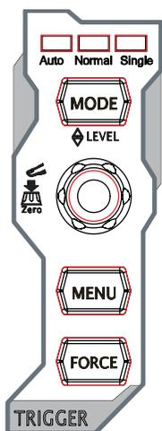
**MODE:** press this key to switch the trigger mode to **Auto**, **Normal** or **Single** and the corresponding state backlight of the current trigger mode would be illuminated.
