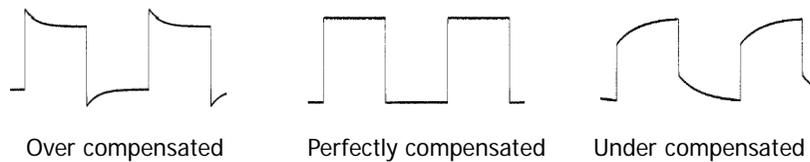
Figure 9 Probe Compensation
