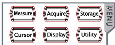
**Measure**: press this key to open the measurement setting menu. You can set the measurement source and turn on or off the frequency counter, all measure, statistic function etc.
