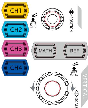
**CH1, CH2, CH3, CH4**: analog channel setting keys. The 4 channels are marked by different colors which are also used to mark both the corresponding waveforms on the screen and the channel input connectors. Press any key to open the corresponding channel menu and press again to turn off the channel.
