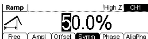
Figure 2-10 Ramp Signal Parameter Setting Interface
