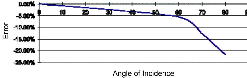
FIGURE 8-2. Cosine response of a typical net radiometer
