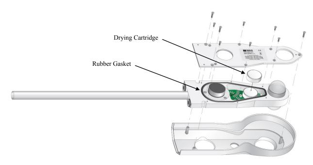
FIGURE 9-1. Replacing the drying cartridge
