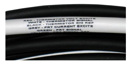
FIGURE 7-4. Labels on the pigtail end of the TEMP cable.
