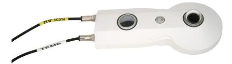
FIGURE 7-1. The CNR4 sensor with SOLAR and TEMP cables
