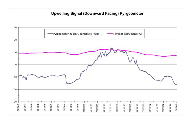
FIGURE C-3. Clear day for the downward facing pyrgeometer
