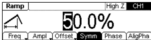
Figure 2-10 Ramp Signal Parameter Setting Interface
